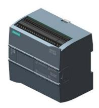
SIMATIC S7-1200, CPU 1214C, compact CPU, AC/DC/relay, onboard I/O: 14 DI 24 V DC; 10 DO relay 2 A; 2 AI 0-10 V DC, Power supply: AC 85-264 V AC at 47-63 Hz, Program/data memory 75 KB
